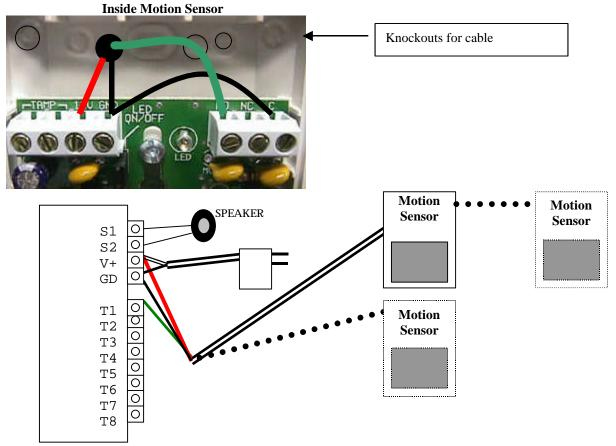
To make sure the motion sensor does not keep restarting the WAV audio file (001.wav) while it is playing, the MODE.TXT file should contain:
