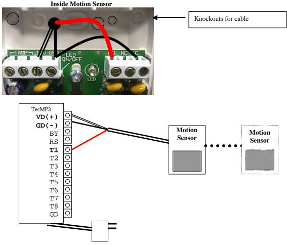
To make sure the motion sensor does not keep restarting the MP3 audio file (001.MP3) while it is playing, the MODE.TXT file should contain:
