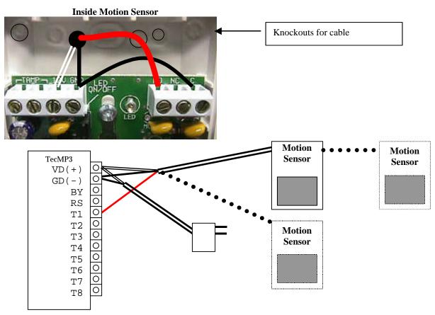
To make sure the motion sensor does not keep restarting the MP3 audio file (001.MP3) while it is playing, the MODE.TXT file should contain:
