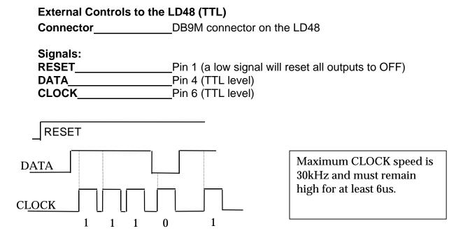
As the data is clocked into the board the bits are shifted each time - the last data bit clocked into the board is always the data bit for terminal 1. For example: if 10 bits are clocked in, the first bit is for terminal 10 and the last bit is for terminal 1. Data is clocked in on the rising edge of the clock line.
